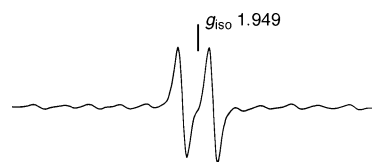
Figure 6. Room-temperature EPR spectrum of [\text{Tp}^*\text{MoO}(\text{S}_3\text{PPr}_2)]^+ prepared by the reaction of \text{Tp}^*\text{MoOS}(\text{S}_2\text{PPr}_2) with excess [\text{FeCp}_2]\text{PF}_6 in \text{THF}/\text{CH}_3\text{CN} (9:1).
